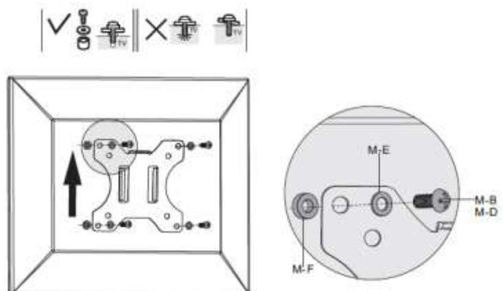
5. Once the plate is fixed securely to the display, re-attach the plate to the mount. When carrying and moving the display and plate, please operate with two people.
