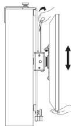
7. To adjust the height of the display, pull the adjustable handle and carefully lower or raise the display to the desired height. Ensure the plate has clicked into place in one of the locking holes for a secure fixing.
